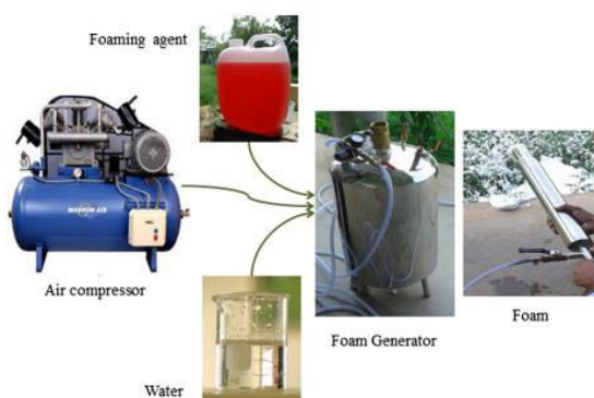
Figure 4: Preparation of foam by the pre-foaming process [2].
